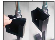
6. Use the large Allen key to tighten the connecting screw bolt.
