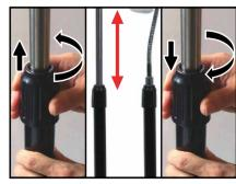
3. Rotate plastic grip counter clockwise to loosen, then adjust pole to desired height. Rotate plastic grip clockwise to tighten.
