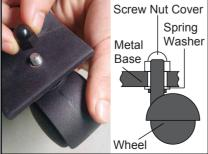
Place the screw bolt from each wheel through the metal base, then place a nut cover over the top of each and tighten until you can not tighten any more by hand. Use the thin wrench to hold the nut cover to tighten further.
