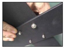
3. Place a washer on the underside of each screw and tighten each up.
