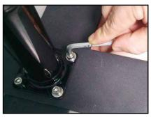
4. Grip the nut on the underside with one hand and use the other to tighten each screw with the Allen key.
