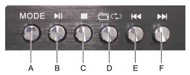
**A. MODE BUTTON:** Press this button to select one from play mode with USB/SD mode, FM mode and Bluetooth mode, automatically set in USB/SD mode after turning on the unit, automatically play mp3 files after inserting a USB flash driver or SD card.
