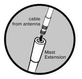
Once you have determined the best location for the antenna and have determined if Mast Extensions are needed, insert cable **through** mast.
