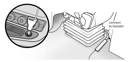
Connect power cable to booster port labeled \_\_\_\_.
