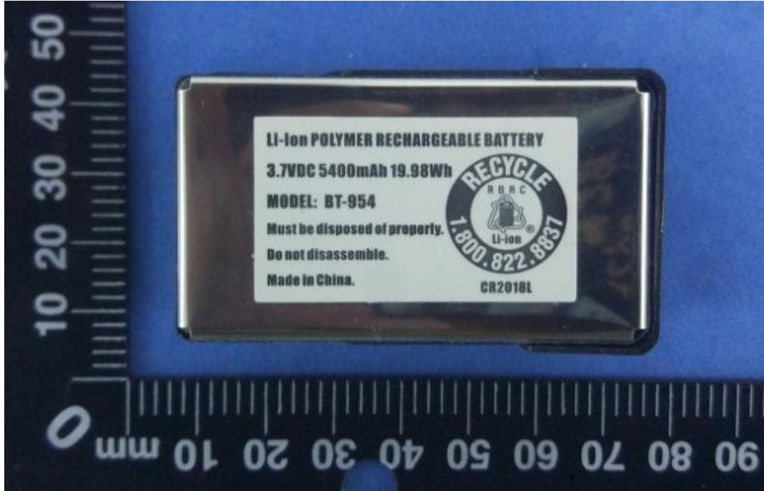
Battery /电池 (BT-954 3.7V 5400mAh 19.98Wh)
