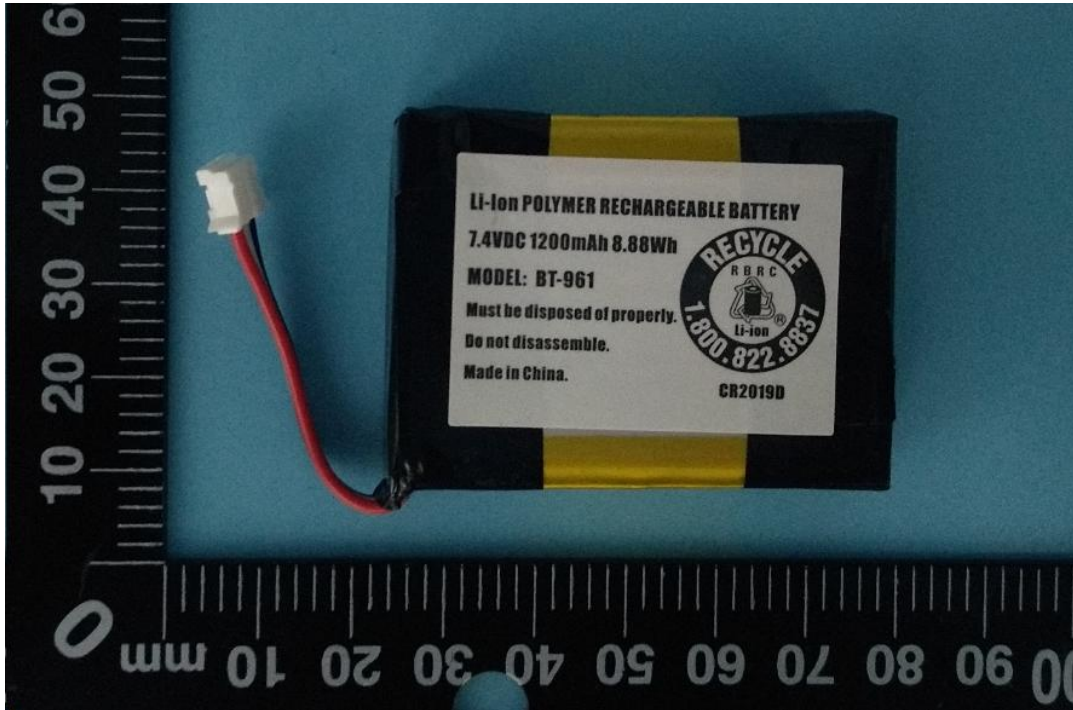
Battery / 电池 (BT-961 7.4V 1200mAh 8.88Wh)
