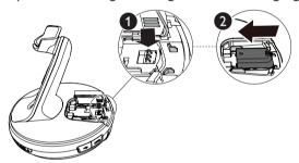
3. Slide the battery compartment cover back to the headset base.
