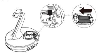
7. Slide the battery compartment cover back to the headset base.
