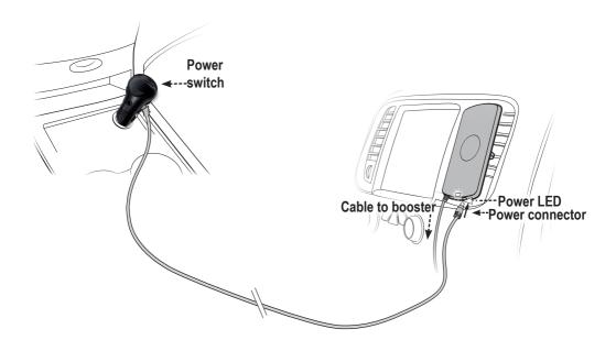
WARNING: The booster is rated for 5-15V input voltage. DO NOT use the booster with a higher voltage power supply. This can damage the booster and/or cause personal injury.
