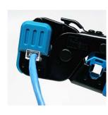
7) Terminate the plug with a modular plug crimper. Use the RJ45 8-position 8-contact cavity.
