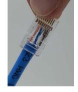
6) Slide assembly into plug body, ensuring conductors are fully inserted to the end of the body.
