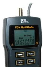
6) Verify correct wiring and termination with a wiremap tester.
