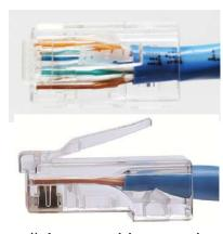
4) Insert cable into plug ensuring conductors are inserted to the end of the connector.
