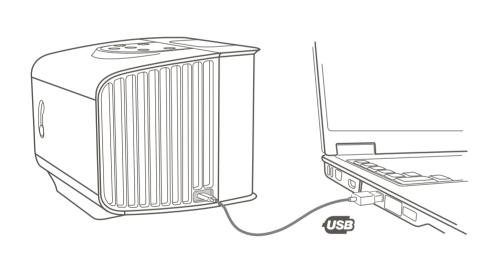
Use the cable to connect the device to the power source: power bank, power socket, laptop, etc.
