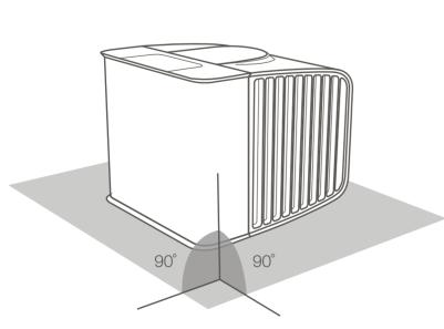
Use the device on the stable and even surface. Do not tilt the device to prevent water leakage and damages. Before movement or transportation, it is highly recommended to empty the reservoir and set the device to run on the maximum fan speed for at least one hour to dry the water out from the internal reservoir.
