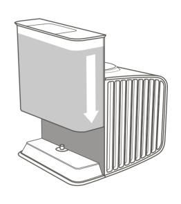
Place the reservoir back onto the base. Make sure it is installed properly.
