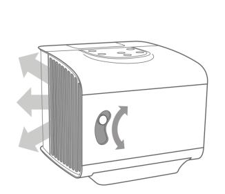
You can adjust the airflow directions by moving the trigger on the side of the device.
