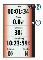
The vehicle position LED ① moves up the column as a vehicle gets closer to your bike. The threat level LED ② changes color based on the potential level of threat. Green indicates no vehicle is detected. Amber indicates a vehicle is approaching. Red indicates a vehicle is advancing at a high rate of speed.
