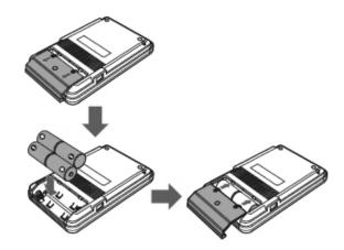
NOTE: Disconnect the AC adapter before installing the batteries.
