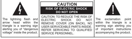
The Caution Marking is located at the bottom enclosure of the apparatus.
