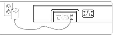
Plug the small end of the power cord into the DC Input on the back of the speaker, and the large plug into a standard wall outlet.
