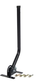
The ClearStream<sup>™</sup> J-Mount is just like our basic J-Mount - only smaller. This 20" mast with a 1" diameter is ideally suited for our ClearStream<sup>™</sup> Antenna line. Like our basic J-Mount, the CS J Mount has a pivoting foot, which allows installation on vertical or horizontal surfaces. Mounting hardware is included.
