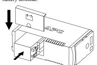
Push the battery into the battery compartment and re-install the cover, as shown.
