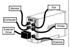
Surge Only Outlets (qty. of 3). These outlets are always **On** (when AC power is available) and are not controlled by the **On/Off** switch. These outlets do not provide power during a power outage. Connect a printer, fax machine or scanner to these out-
