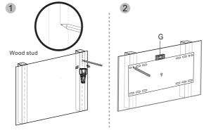
Caution: The minimum size of the woodstud must be 2"x 4" and the thickness of the drywall must not exceed 5/8"
