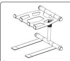
Step 1 To fold stand; extend telescoping neck to appropriate height.
