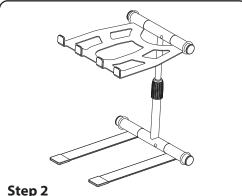
Press retaining pin until legs fold up. Retaining pin should pop into second hole, holding unit legs folded closed.
