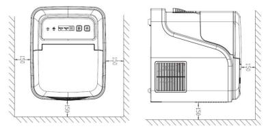
The machine should be upright to place on the horizontal plane. To ensure the machine ventilate normally, it is important to set 150mm room on top, sides and back. Do not place the machine next to the roast oven, radiate or other heat objects.
