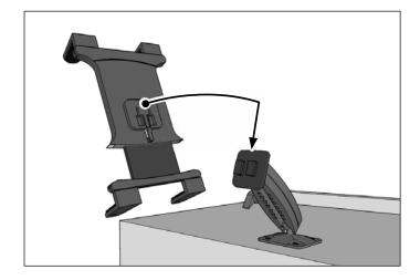
3 Insert tablet by placing it on the two lower legs and pushing down on the spring-loaded bottom of the holder. Loosen adjustment knob to adjust rotation, position, or angle. Retighten to set.
