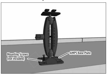
2 Attach Slim-Grip tablet holder by sliding the Dual T-Tabs on the pedestal head into the Dual T-Slots of the holder.
