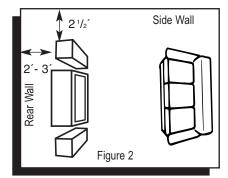
Note: For best results, maintain a minimum distance of  $2\frac{1}{2}$  feet away from the side wall (as shown).
