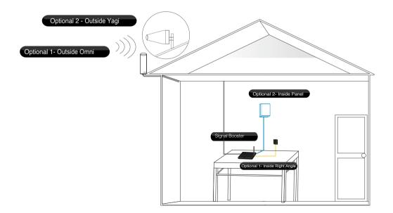
Omni antennas come with equipment for mounting on a vertical wall. For best results the antenna should be mounted in an upright position.
