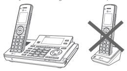
For registration, put the handset on the telephone base, not the handset charger.
