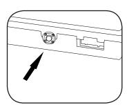
Press the programming button on the side of the interface while OnStar is active to adjust the OnStar volume
