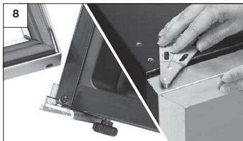
To reattach the door, place the door onto the bottom axle insert. Place the top **bracket** into the door and align the metal **bracket** holes over the holes in the top of the unit cabinet. Tighten the three screws to hold in place.
