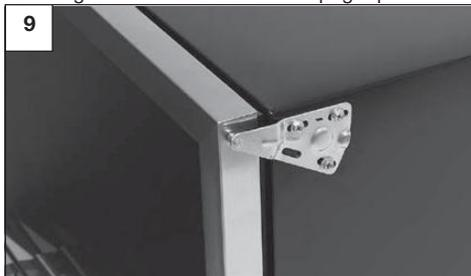
The rubber gasket should be compressed on all sides of the door. If the gasket is more compressed on one side, the metal bracket position should be adjusted. Make sure the door is level. Once the door position is finalized, securely tighten the screws.
