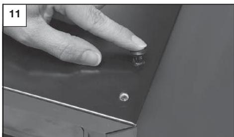
Reinstall all plastic **hole insert plugs**. The re-installation of the plastic **hole insert plugs** is important to maintain the seal and integrity of the insulation. Extra inserts are included in case the plugs are damaged during removal.
