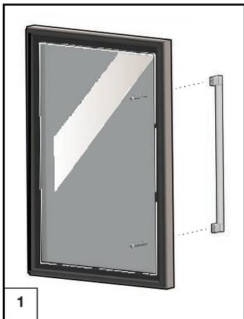
The stainless steel handle is easily attached to the left side of the glass door with two enclosed screws.
