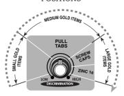
The illustration above shows the approximate positions where different types of metals are eliminated. Objects come in many shapes, sizes, and levels of purity, so these positions can vary.
