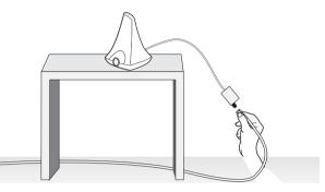
Placing Booster and connecting cable
