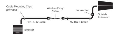
Route cable to the **Home MultiRoom Booster** and connect to the port labeled 'OUTSIDE ANTENNA'.
