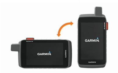
**NOTE:** While using the inReach features of your Montana 700i/750i device, you should use the device in vertical (portrait) mode, with the antenna pointed toward the sky.
