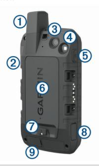
1 Iridium® and GNSS antenna SOS button Camera lens (Montana 750i only) Flashlight Camera flash (Montana 750i only) Power button **(5)** 0 6 microSD® card slot (under battery pack) Battery pack D-ring 8 Micro-USB port (under weather cap) 9 External Iridium and GNSS antenna port (under weather cap)
