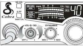
3 To achieve the Desired Squelch Setting (DSS), turn the Squelch control *counterclockwise* until you hear noise. Now turn the control *clockwise* just until the noise stops. This is the DSS setting.
