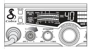
1 Rotate the **On/Off Volume** knob *clockwise*. The RX icon will be displayed.
