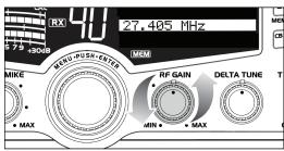
• Rotate the RF Gain knob counterclockwise to reduce gain in strong signal areas. In weak signal areas turn clockwise to increase gain.
