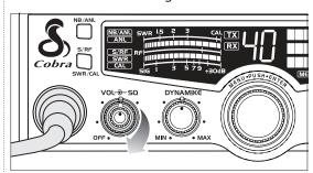
• Rotate the **On/Off Volume** knob *clockwise* to turn unit on and adjust to a normal listening level.
