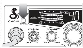
The S/RF-SWR-CAL button must be in the S/RF mode.
