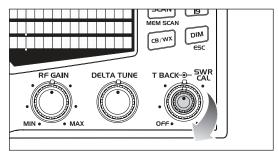
While holding mic button adjust the SWR CAL knob so the meter swings to the CAL mark on the meter (located on the right).
