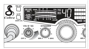
2 Full counterclockwise rotation opens the "gate" allowing all signals in.
