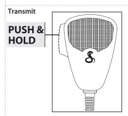
Push and hold mic button to transmit. Transmitter is now activated. When transmitting, hold the microphone two inches from your mouth and speak in a clear, normal voice. Release to receive.
