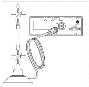
3 Connect the antenna cable plug to the receptacle marked "ANT" on the back of the unit.
