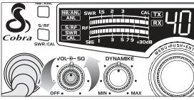
3 To achieve the Desired Squelch Setting (DSS), turn the Squelch control *counterclockwise* until you hear noise. Now turn the control *clockwise* just until the noise stops. This is the DSS setting.
