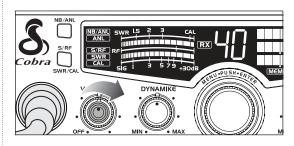
• Rotate the **On/Off Volume** knob *clockwise*. The RX icon will be displayed.
