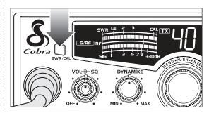
The S/RF-SWR-CAL button must be in the S/RF mode.
