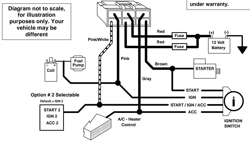
\*\*\* Fuse Holders Wire Connections should NOT GET HOT \*\*\*
