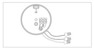
Place the back plate against the outlet box, insert the mounting bracket screw through the back plate hole, thread mounting bracket screw into the center hole of the mounting bar. Tighten the mounting bracket screw securely. Note: The "UP" arrow must point upward.
