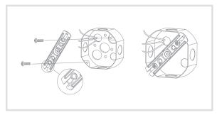
2 Unscrew the center mounting screw on the light fixture in order to remove the back plate on the back of the light fixture
