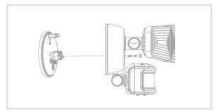
Connect the source wires from the outlet box with the wires of the back plate using wire nuts as follows: Connect the white wire to white wire Connect the black wire to black wire Connect the Green wire to the house ground wire Note:
