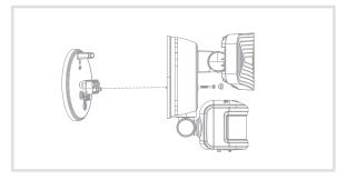
3 Connect the source wires from the outlet box with the wires of the back plate using wire nuts as follows:
