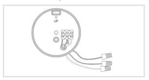
4 Place the back plate against the outlet box, insert the mounting bracket screw through the back plate hole, thread mounting bracket screw into the center hole of the mounting bar. Tighten the mounting bracket screw securely.
