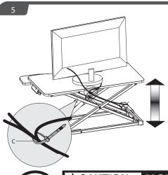
Use the plastic wire tie (C) to finish securing the wires and cables for all your devices. Be extra careful to allow for the movment of the desk surface. Allow enough slack in the wires and cables so as not to get pinched or trapped in the armature of the SD320.
