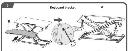
Position keyboard table (B) on to the keyboard brackets on main unit (A). Thread the four screws (D) through the keyboard brackets into the keyboard table. Tighten the screw using the supplied tool (G)
