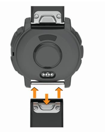
**NOTE:** Make sure the band is secure. The latch should close over the watch pin.
