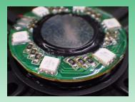
Water-resistant coating has been applied to LED's printed circuit board.
