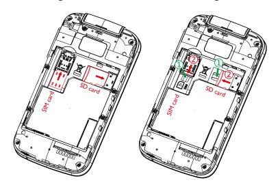
To remove the SIM card or microSD card, press down on the small plastic tab (1), then slide out the card (2). Do not use force or any sharp objects.
