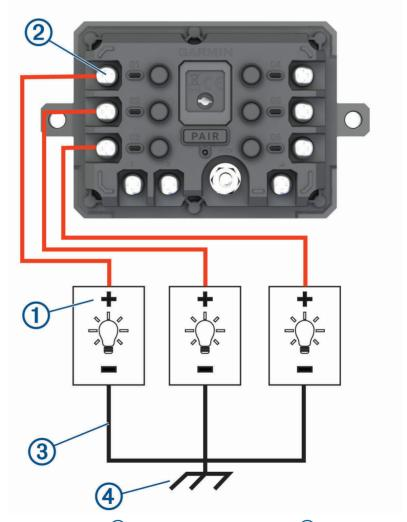
2 Connect the negative or ground wire 3 to an unpainted ground stud 4 on the vehicle frame, to a ground distribution block, or directly to the negative terminal on the battery.
