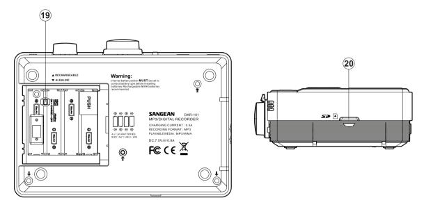
19. Alkaline/NiMH/NiCad rechargeable battery switch
