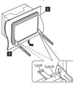
2 When the lower level is removed, remove from the upper two catches of the trim plate (6).
