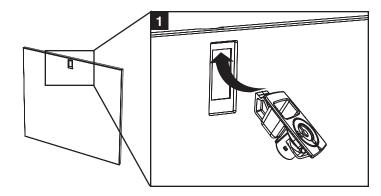
**2** Push the lower portion of the latch into the side panel cutout as shown.
