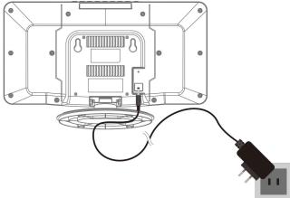
To do this, place the connection cable plug in the socket DC IN and the supplied mains adapter into a properly installed earthed power socket which is accessible at all times
