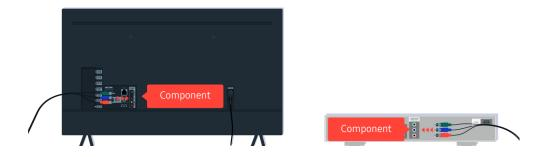
If a component cable is used, make sure that the colored connectors are connected to the matching connectors on the external device and the TV.
