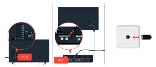
Check the antenna and input cable connections.
