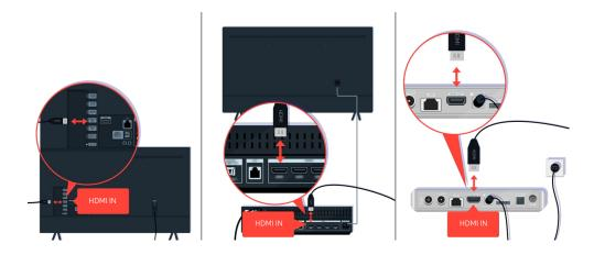
Check the antenna and HDMI cable connections.
