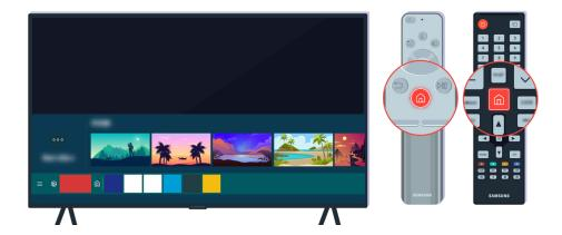
On the remote control, press the 🚳 button. When the Home Screen appears, the TV is turned on but the connected external device does not work or any connection problem occurs.
