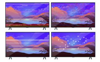
If the issue persists, define exactly what is wrong with the display. For example, mosaics and blocks, multiple lines or white dots, fixed horizontal, or vertical lines.
