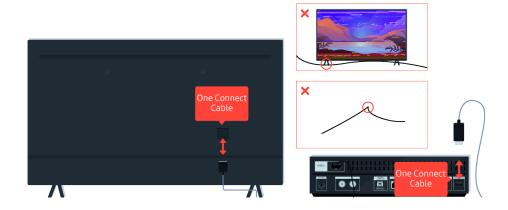
If the problem persists, and if your TV uses the One Connect Cable, disconnect and reconnect the One Connect Cable to the TV and the One Connect (OC) Box. Ensure that the One Connect Cable is not pinched or bent sharply.
