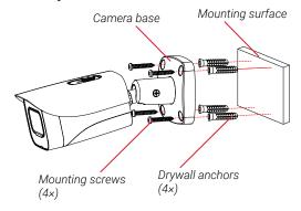
1. Use the included mounting template to mark holes for the screws. Drill holes for the mounting screws.
