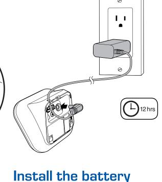
1. Plug the battery connector securely into the socket inside the handset
