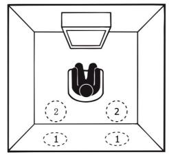
Acoustech ceiling speakers may be used for surround and rear sound channels by placing them (1) behind or (2) in the ceiling, just behind the viewer.
