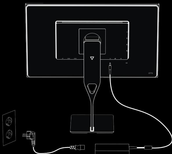
Connect the power cord to the AC adapter and plug the other end into a grounded AC outlet. Then connect the AC adapter to the power connector on the rear of the monitor.
