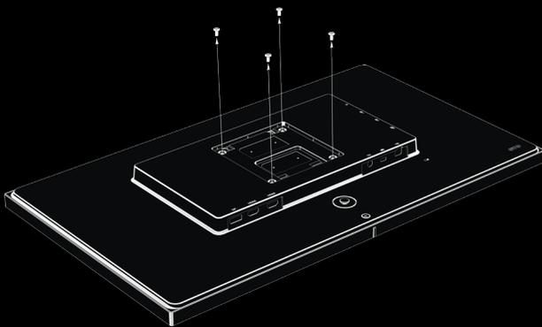
Remove the four mounting screws from the back of the monitor.
