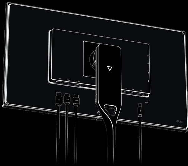
Connect an HDMI or DisplayPort cable to one of the ports on the rear of the monitor, and the other end to the source device. Then connect a USB cable to the USB Type-B upstream port on the rear of the monitor, and the other end to the host device.
