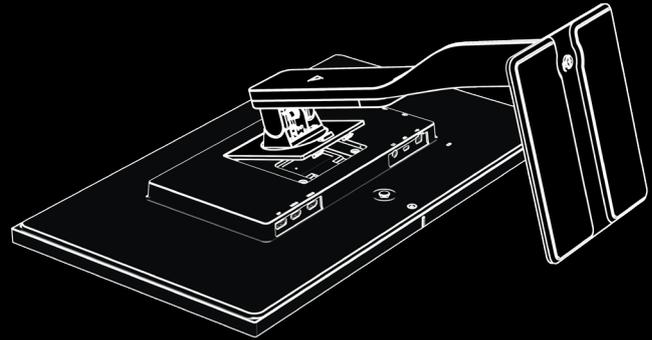
Insert the top of the stand into the back of the monitor cabinet at an angle, then press down. The stand will click into place.
