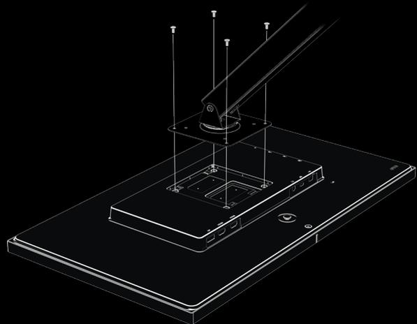
Align the screw holes on your mounting device with the four VESA screw holes in the back of the monitor, then insert and tighten the four mounting screws through the mounting device and into the monitor.
