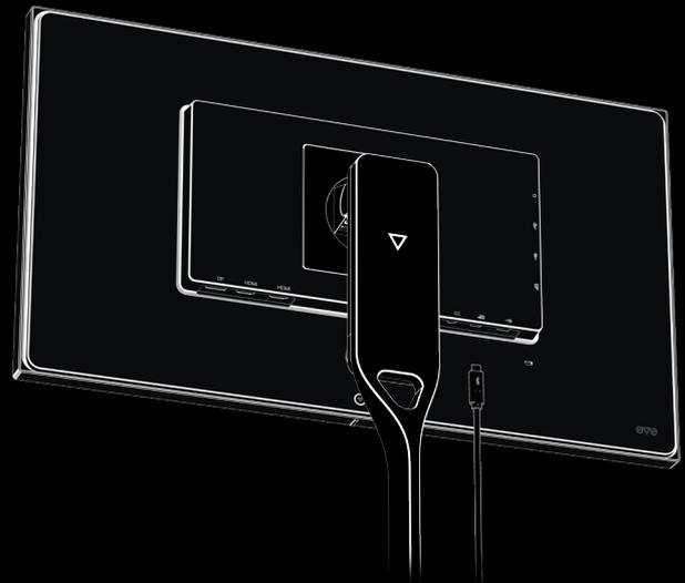
Or: Connect a USB Type-C cable to the bottom USB Type-C port on the rear of the monitor, and the other end to the source device. Your device must support DisplayPort Alt Mode for video output, and USB Power Delivery for charging.
