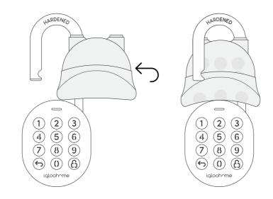
Pull and fold the silicon case down to ensure it covers the whole padlock.
