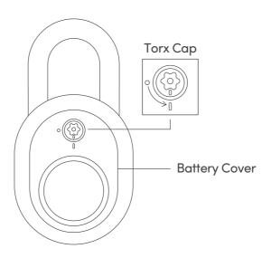
Please ensure battery is inserted into the Padlock and Torx cap is in locked position with the battery cover closed before putting on the Silicone Case.
