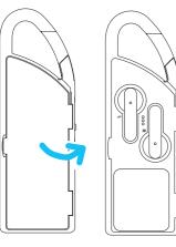
Insert the provided charging cable into the charging jack on the side of the speaker. Plug the other end of the charging cable into a USB power source (like a computer or a USB charger).
